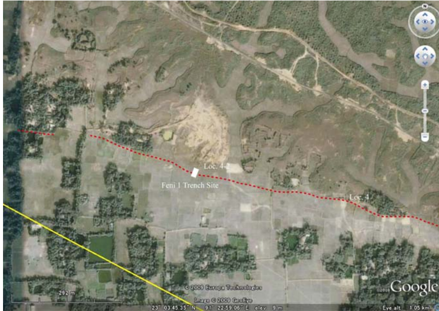
Figure 3-9 Inferred active fault trace in Loc.4 and Loc.4-2. Background is Google Earth image.
