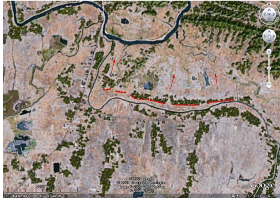
Figure 3-16 Inferred active fault trace in the northeast of Sylhet. Arrows represent back-tilting surface. Background is Google Earth image.
