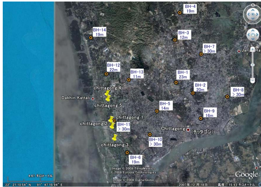
Figure 3-6 Drilling data in Chittagong. The top and bottom in the rectangles represent the number of drilling and the depth of the top of the Tertiary sediments, respectively. Data was offered with courtesy of GSB.
