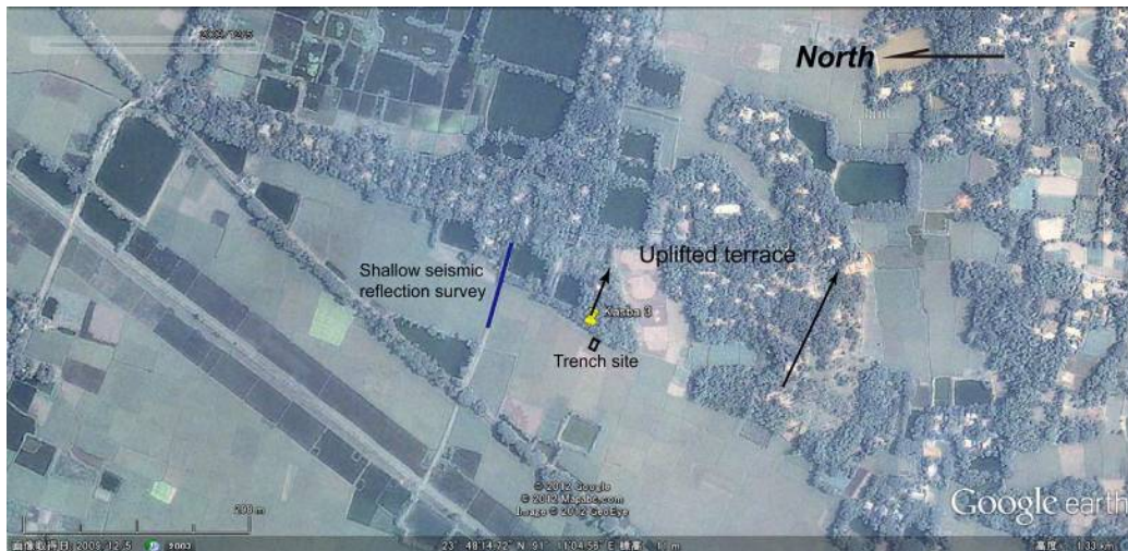
Figure 17. Back-tilted terrace at Kasba. The arrows represent back-tilted surface. A shallow seismic reflection survey is planned.
