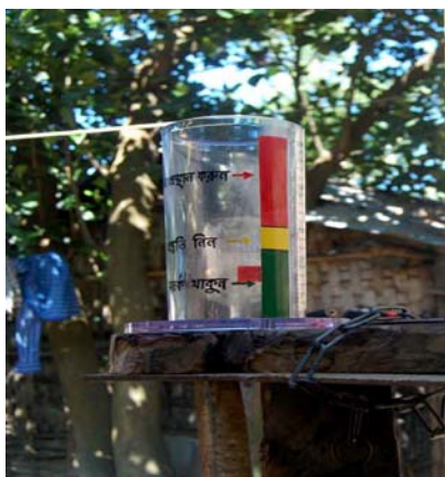
Rain Gauge Installed in a Community at Cox's Bazar
