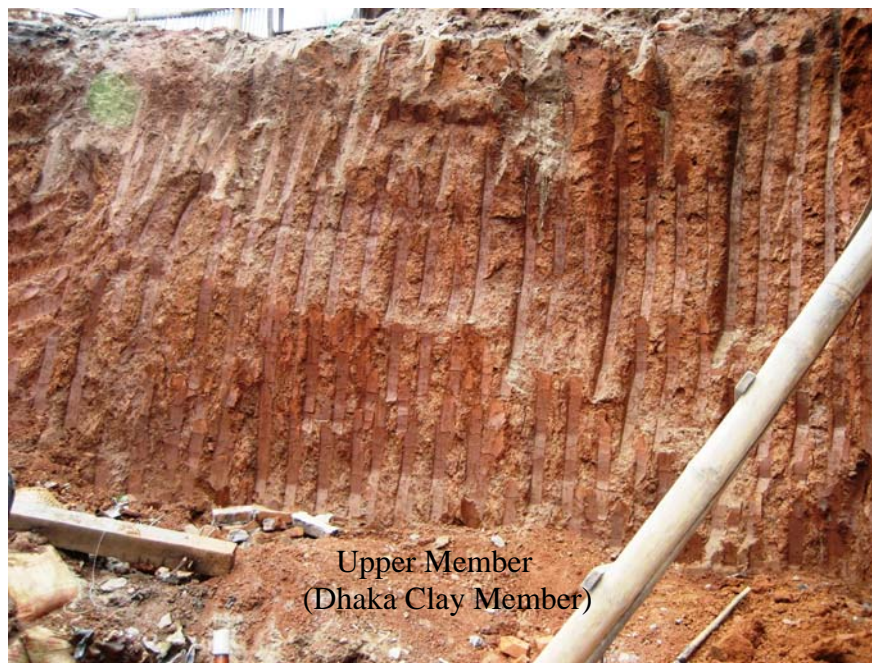
Photo-2.17. Shows the intense weathering of the Upper Member of Madhupur Formation. Section at Mirpur-1, Beside Muktijadhay Supper Market, Dhaka City.
