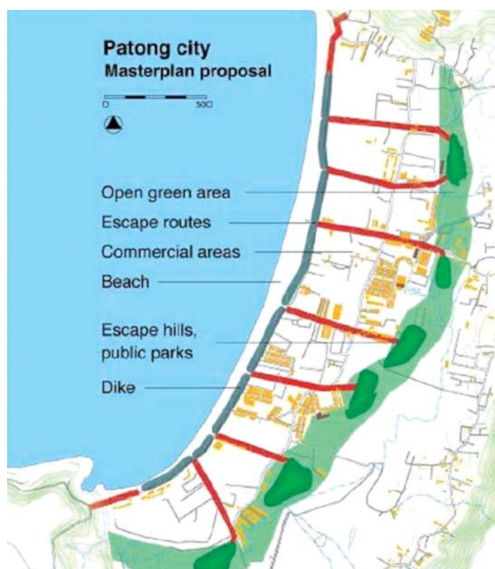
Fig 4: Mitigation Master plan for Patong, Phuket was introduced as the example for populated tourist area (CCOP, 2006a)
