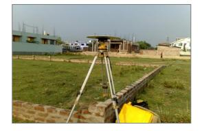
Geo-Referencing of Image using RTK GPS
