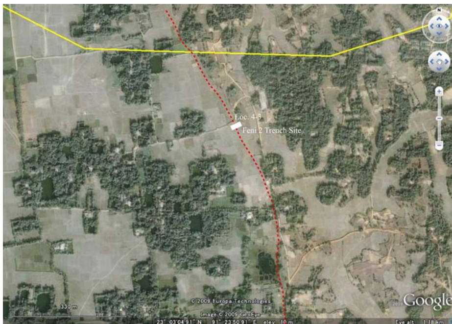
Figure 3-10 Inferred Active Fault Trace in Loc.4-3 (Background: Google Earth)
