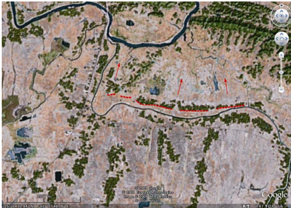
Figure 3-16 Inferred Active Fault Trace in the Northeast of Sylhet
