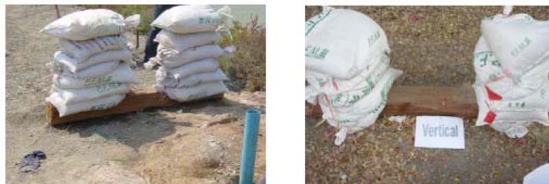
Figure 2-4 Wooden Plank as the Vibration Source
