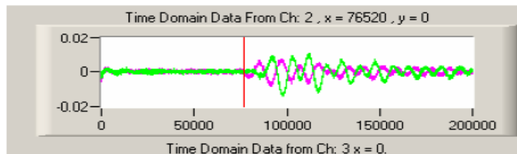
Figure 2-10 Determination of the Arrival Time of S-wave
